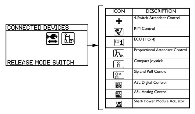
FIGURE 5.7 LCD Display Screens - Connected Devices Screen
